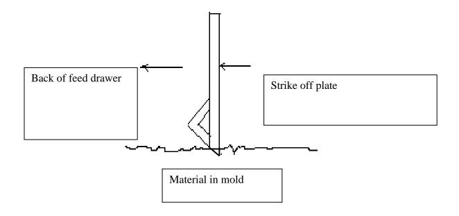
h. Weld 1/8" – 3/16" / 3-5mm thick flat bar in staggered heights to the fingers of the agitator. These will act as secondary strike of bars and help the final strike off making a more even pass by limiting the amount of material to strike off.
